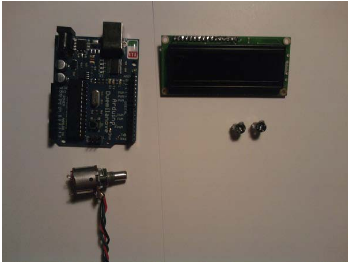
Figure 4-4. Hardware for this project (Not pictured: the USB cable, extra wire, and solderless breadboard)
