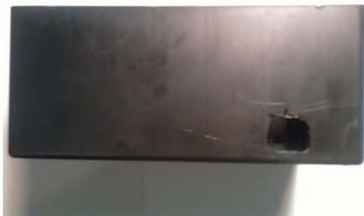
Figure 8-7. Drill a hole so that power can be connected to the Arduino.
