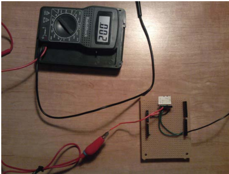
Figure 11-23. Checking whether two terminals are connected; if the multimeter displays “OL,” then the terminals are not connected, which could be an issue.
