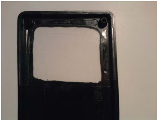
Figure 6-10. Clear screen attached with double-sided tape
