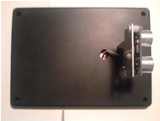
Figure 8-6. Attach ultrasonic sensor to bracket.
