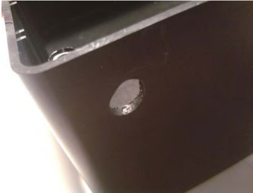
Figure 9-6. Modify enclosure so that it can hold the duck antenna.
