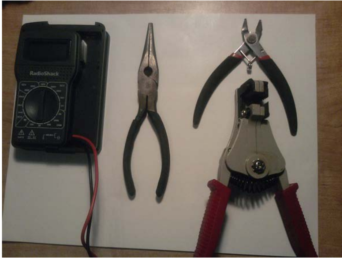
Figure 1-9. Additional Tools from left to right: multimeter, needle-nose pliers, wire clippers (top), wire stripper (bottom).
