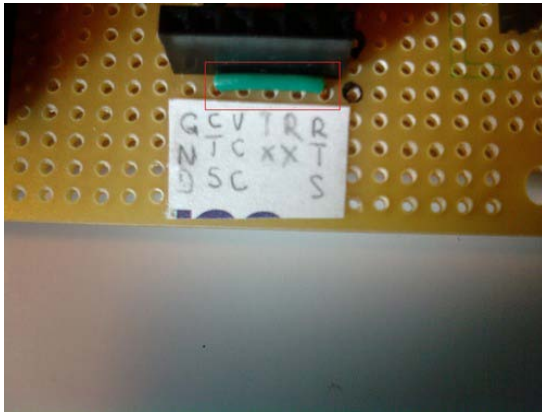
Figure 11-9. Solder the CTS and RTS pins together from the 6-pin header.
