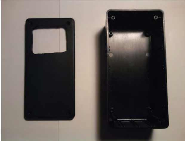
Figure 6-9. Square cut out of the lid of the enclosure
