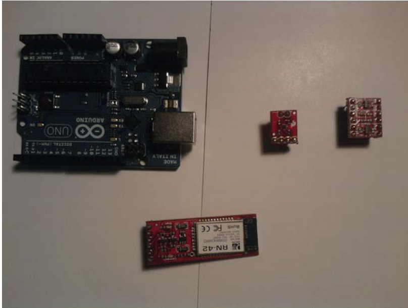
Figure 6-22. Hardware for this project (Not pictured: solderless breadboard, 9V battery, 9V battery connector, and extra wire)
